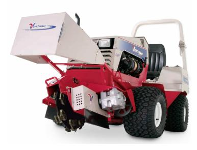
The KC180 Stump Grinder makes quick work of unwanted stumps and roots. Heavy-duty carbide cutters provide extended and effective performance in spite of dirt, stones, and debris in work area.
