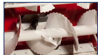
Double spiral serrated auger
