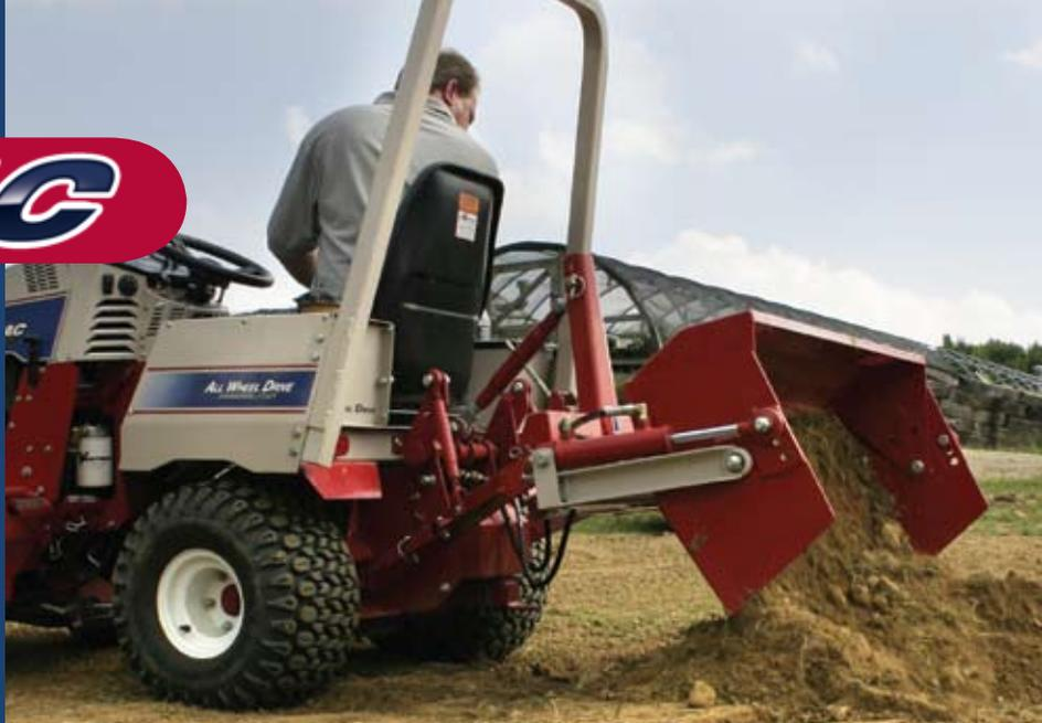
**Connect to the front or rear:** The Ventrac excavator buckets can be mounted to the rear of Ventrac 4000 series tractors equipped with a three point hitch and 3-N-1 Adapter.
