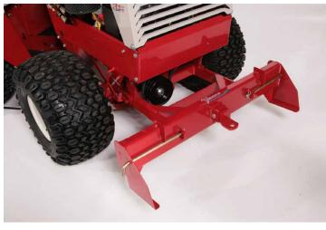
The 2-N-1 fits the front of either 3000 or 4000 series tractor and combines the 2 inch receiver tube for towing with a Front Counter-Weight Bracket capable of holding six 42 lbs (19 kg) weights.
