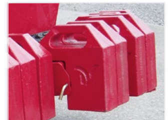
Weight extension bar for mounting four extra weights
