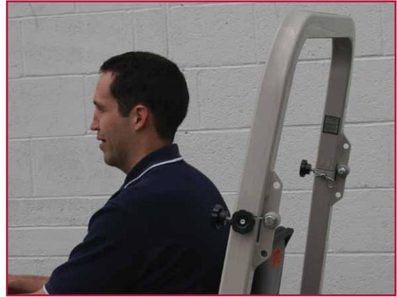
The Fold Down Roll Bar is ideal for operating your tractor in situations where a standard roll bar would obstruct operation, such as under low-hanging trees or in low-clearance areas. Always stop and place roll bar back in its upright position once you have passed under any low obstacle to ensure safe operation.
