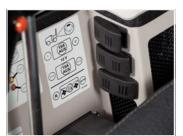
The optional 12 Volt Rear Plug provides power to the rear of Ventrac 4500 Tractor and is required for the Spreader 220. Switches to engage the 12 Volt Rear Plug are conveniently located next to the S.D.L.A. Handle.
