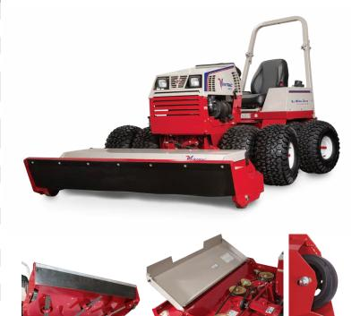
The HQ680 Tough Cut is designed for mowing high grass, thick weeds, and heavy brush. A large baffled front opening directs material into the deck and helps hinder debris from escaping.
