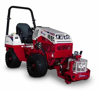
The KA160 Power Blower features a vertical shaft design that delivers a powerful, yet quiet performance. It can be used to remove leaves, light snow, water, and other debris.
