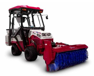
The KJ520 Power Broom is optimized to handle a wide variety of snow on sidewalks. With a higher tip speed and increased hydraulic capacity, this broom can clear snow where other brooms struggle.
