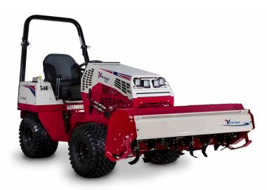
The KL480 Tiller is designed for easy preparation of gardens and yards. This power-driven front-end attachment allows the operator to easily monitor the tiller's performance. Designed with the Ventrac Mount System, the tiller can be attached in a minute or less and comes with a stand for storing when not in use.
