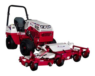
Ventrac's Contour Mower features a 83-inch working width making quick work of any mowing job regardless of the terrain without sacrificing quality of cut. Three independent decks aided by front rollers float along the contour of the ground providing an even cut without scalping, while the rear rollers leave behind a beautiful finish striping pattern. The Contour Mower also features a flip-up deck design.
