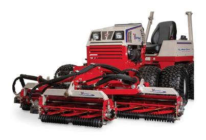
Length 48 inches (122cm) Width 84 inches (214cm) Height 22 inches (56 cm) Weight 613 lbs (278 kg) Shipping Dimensions (LWH) 55x48x45 inches (140x122x114 cm) Reel Specifications Reel Drive Hydraulic Reel Speed Variable Back-lapping Standard, with Individual Bypass Valves 3 **Cutting Units** Reel Length 26 inches (66 cm) Reel Diameter 7 inches (18 cm) Reel Blades 7 Reel to Bed knife Adjustment
