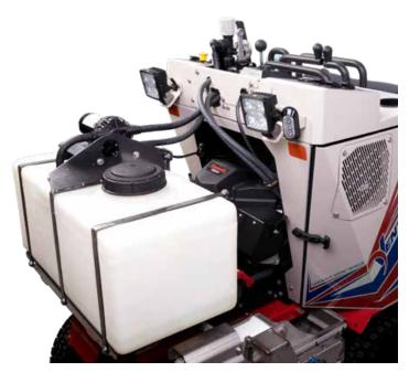
The NB200 Brine Kit features a 20 gallon tank, rear mounted nozzles, and a spray wand. The nozzles distribute brine in a 36" - 48" spray pattern. The optional wand features a coiled hose for easy storage and operation.
