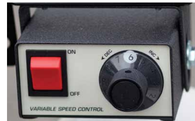
Variable Speed Electronic Controls.
