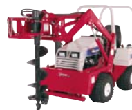
POST HOLE DIGGER Fast drive motor
