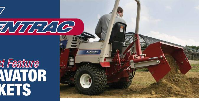
**Connect to the front or rear:** The Ventrac excavator buckets can be mounted to the rear of Ventrac 4000 series tractors equipped with a three point hitch and 3-N-1 Adapter.
